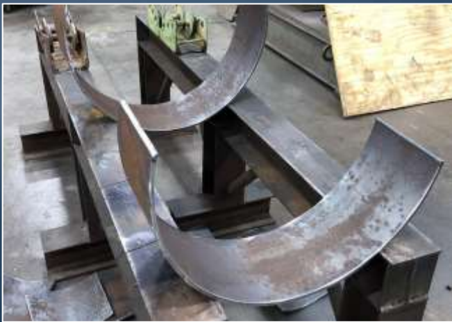
Butt strap joint fabrication (left) and materials and hardware (right) to be provided to SCWD
