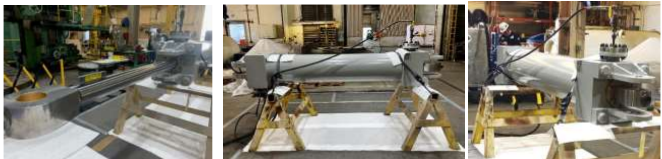
Staff performing functional test (left), hydrostatic test (center), and leakage test (right) of actuator for DWR
