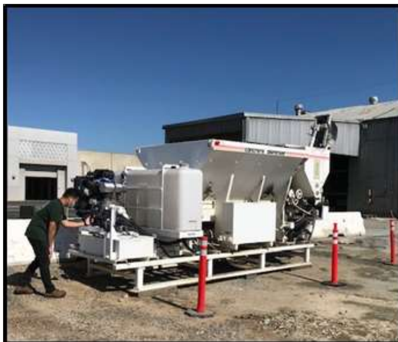
SCAQMD remote inspection of concrete dispenser labels at the Weymouth plant
