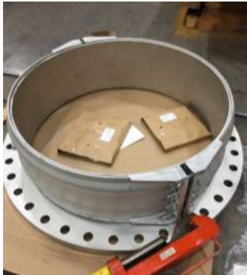
Victaulic coupling test fitted on the thimble for West Valley Feeder No. 1
