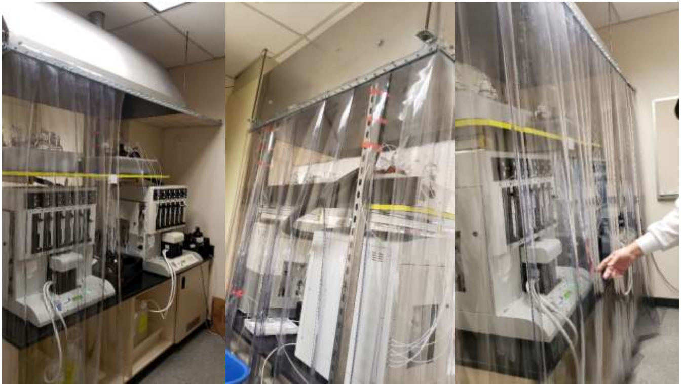
Clear vinyl curtain installed over sampling station in the Water Quality Laboratory
