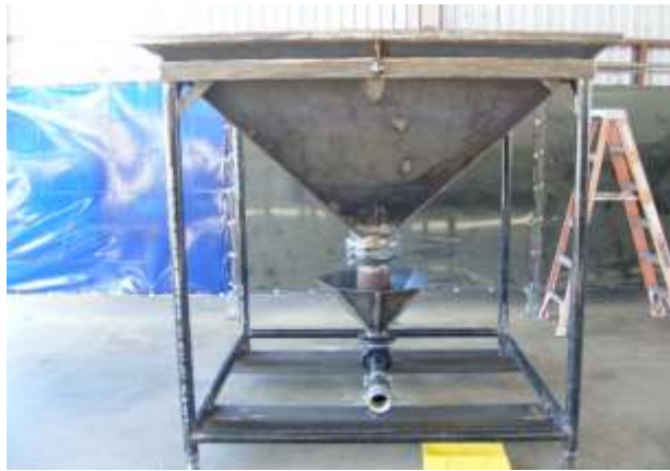
New filter media hopper for the Jensen plant
