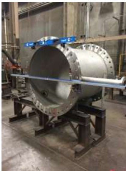
Flanges, drain, and sample lines being fit to a pipe section for West Valley Feeder No. 1
