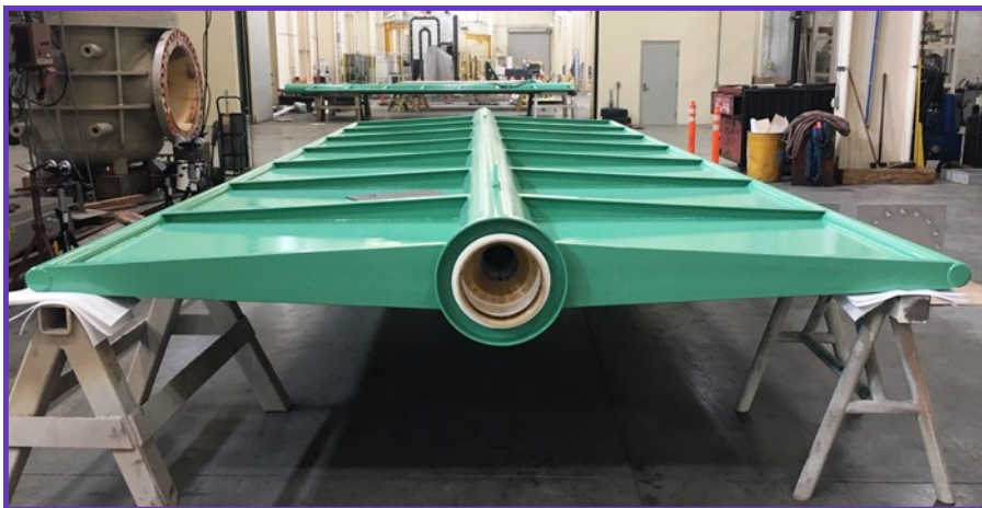
DWR wing gates after manufacturing and coating at the La Verne Shops
