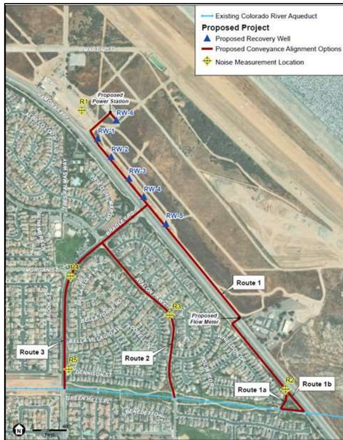
Proposed seepage recovery system alignment
