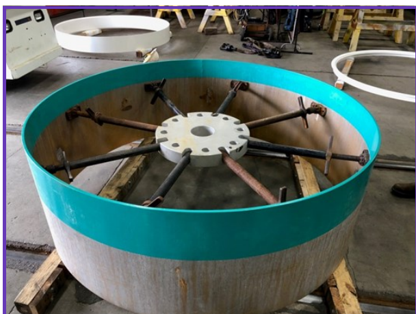
Newly manufactured 79-inch diameter replacement spool
