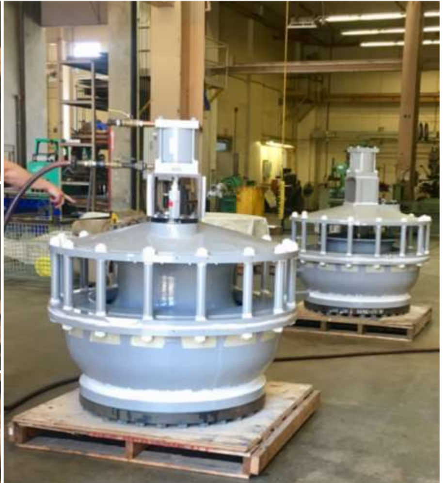
Refurbished Siphon Breakers for Dos Amigos Pumping Plant
