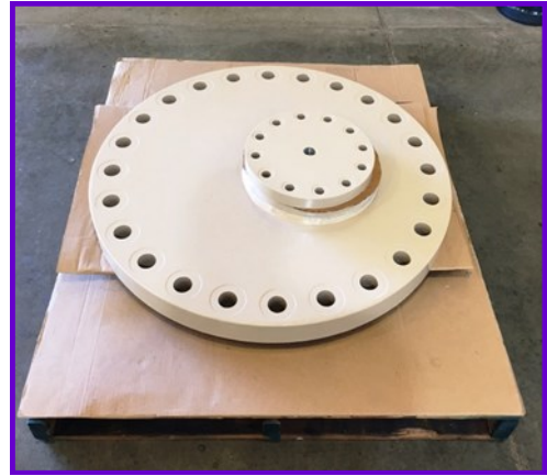
The new 300-pound, 24-inch by 36-inch outlet tee (left); and (right) offset adapter flange with 6-inch blind flange manufactured and coated by the La Verne Shops for the Orange County Feeder Relining Project.
