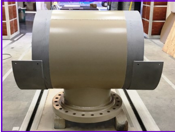
The new 300-pound, 24-inch by 36-inch outlet tee (left); and (right) offset adapter flange with 6-inch blind flange manufactured and coated by the La Verne Shops for the Orange County Feeder Relining Project.
