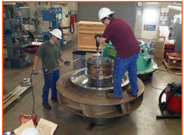
Removal of rotating sleeve for Pump Unit # 3 at Intake Plant.
