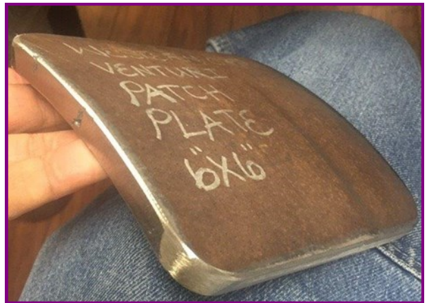
Patch plate to be welded over pinhole leak on venturi meter
