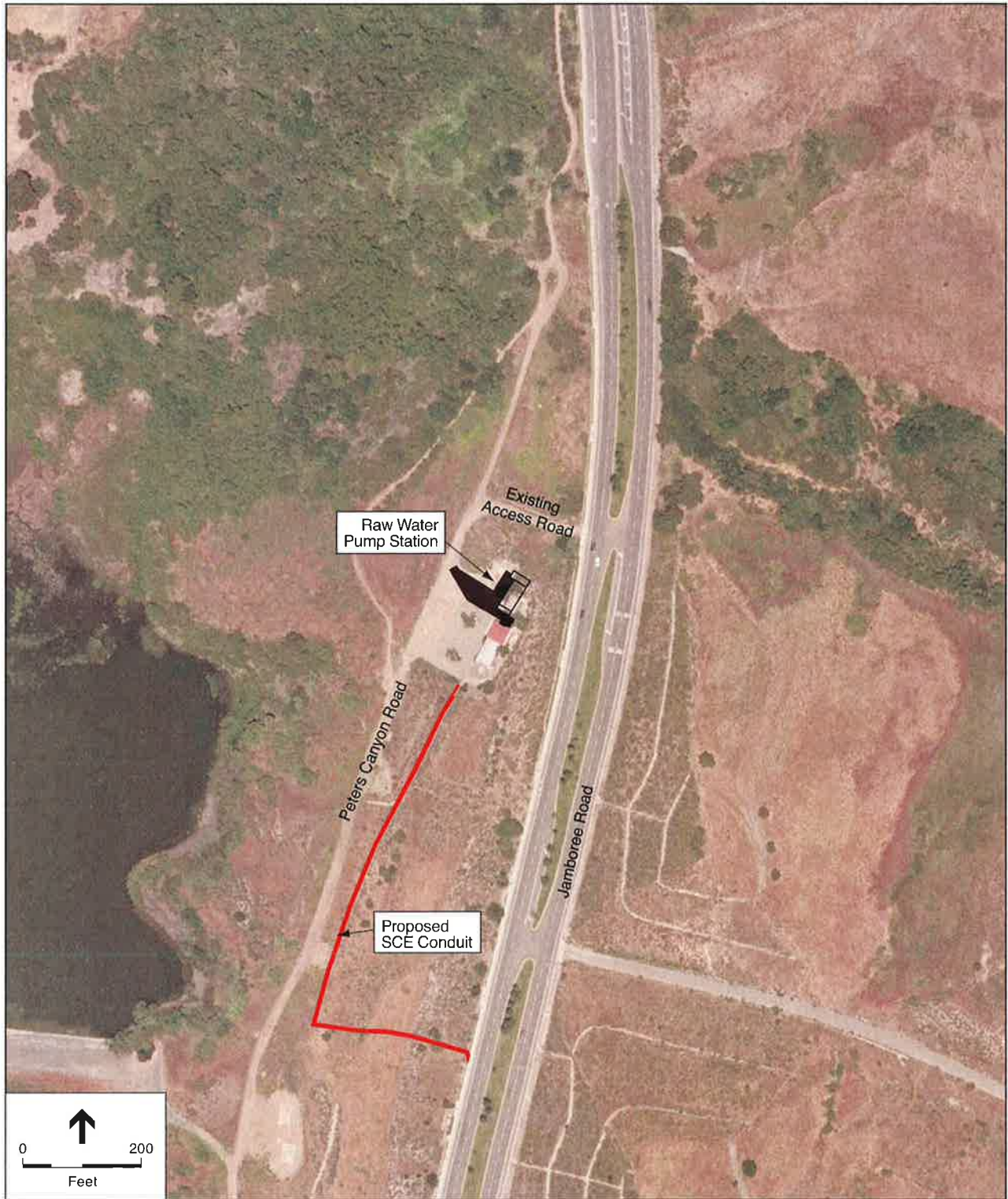
Figure 2 Raw Water Pump Station Proposed Modifications
