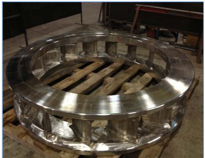
New stainless steel turbine runner
