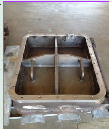
Gianelli scroll case access door after fabrication and before coating operations
