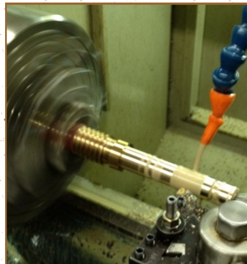
New valve operator shaft being machined at the La Verne Machine Shop. The orange arm is applying a lubricant to the cutting tool.
