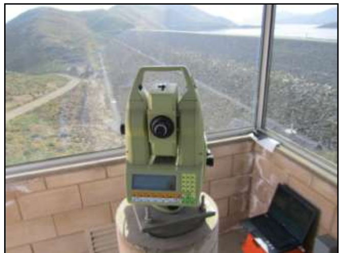
Automated Dam Monitor at Diamond Valley Lake
