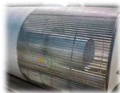
Seawater desalination intake test screen
