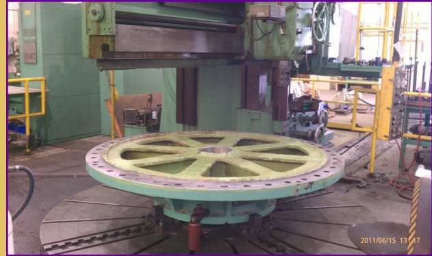
Eagle Mountain Pumping Plant Unit 1 Discharge Valve Rehabilitation at the La Verne Machine Shop.
