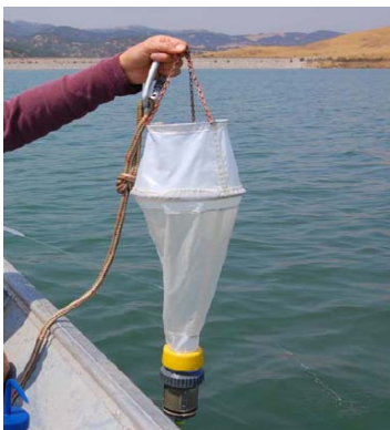
Figure 5 Testing for mussel veligers (larvae) (DWR photo.)
