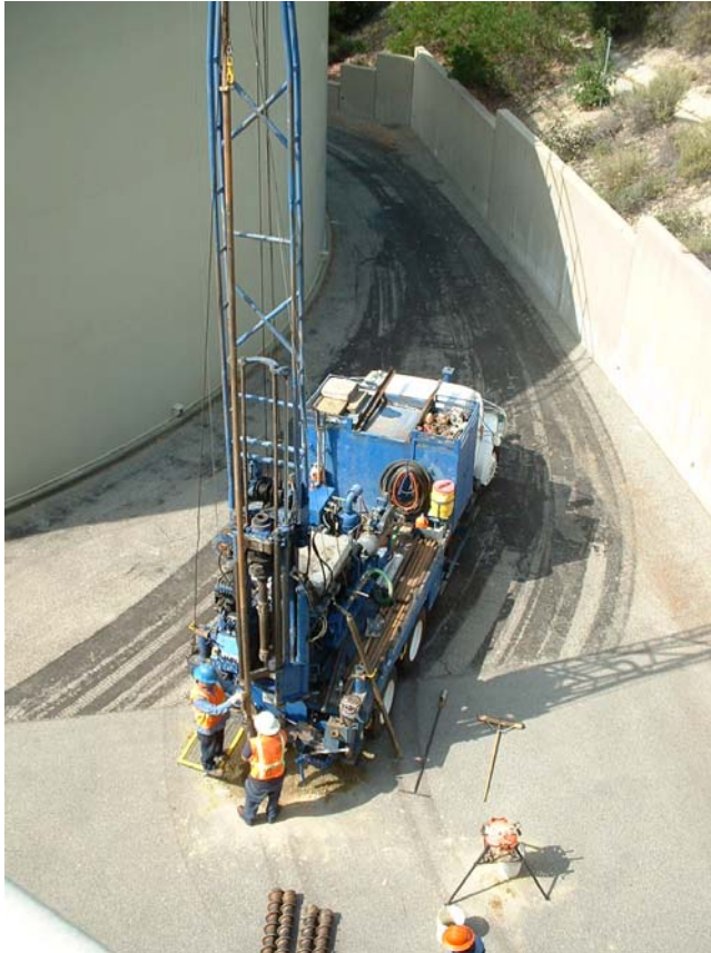
Figure 9: Soils boring adjacent to washwater tank at Jensen plant
