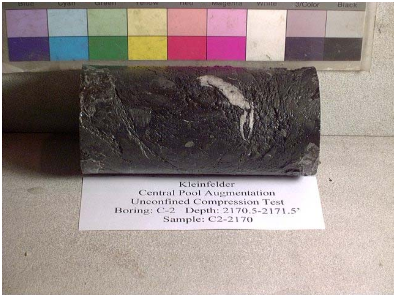
Figure 2: A core sample taken from Boring C-2 on the CPA tunnel alignment
