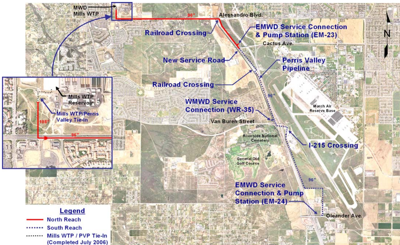
Figure 4: Perris Valley Pipeline Alignment
