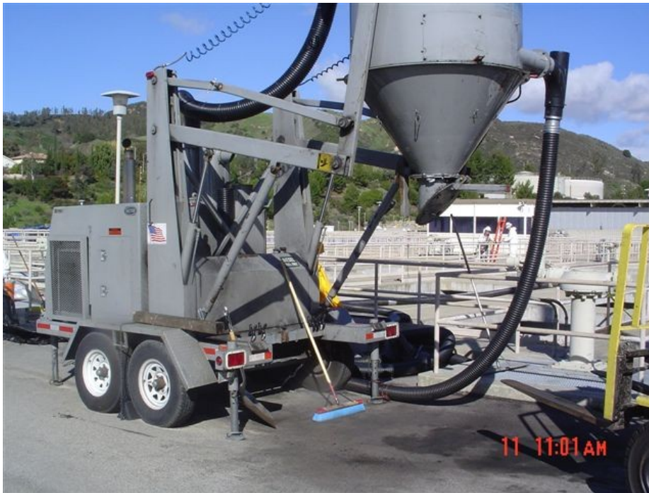
Figure 6: Filter media vacuum truck
